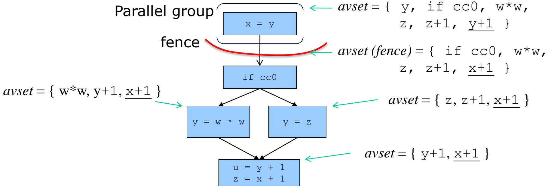
CFG traversed from the top and if current form of expression is in the successor's  $av\_set$ , we check the register availability on the code motion path. Register  $z$  is unavailable, so we choose  $z'$ .
