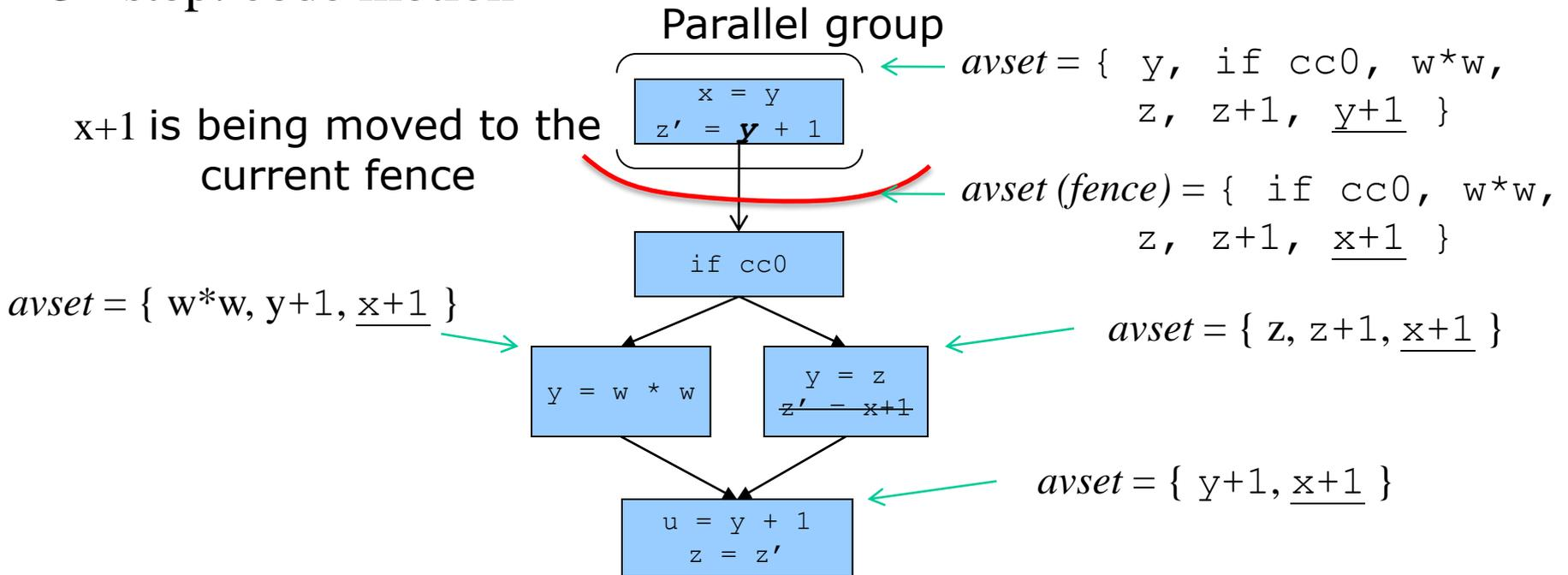
CFG traversed the same way as on previous step. This time we create bookkeeping on the join points, which later might be removed, if the operation is also available on that path
